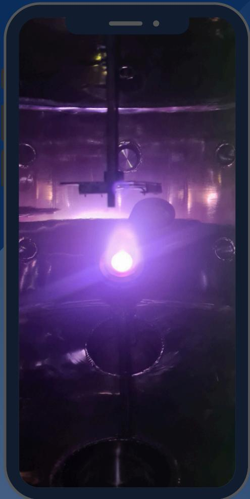
Distinct plasma color and emission intensity profiles illustrate the material-dependent ionization efficiency. The HiPulse modulation system ensures stable discharge conditions, minimizing arcing and improving film uniformity.
